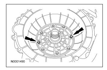
Apply petroleum jelly to the locknut seal.
